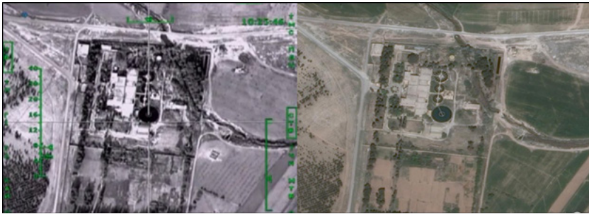
Satellite imagery from Google Earth (right) reveals that the supposed oil refinery near Khafsa Kabir, Syria (left), is actually the Al-Khafsa water treatment facility, located at 36.178345, 38.041224. Photo: (left) Russian Ministry of Defense, (right) Google Maps
